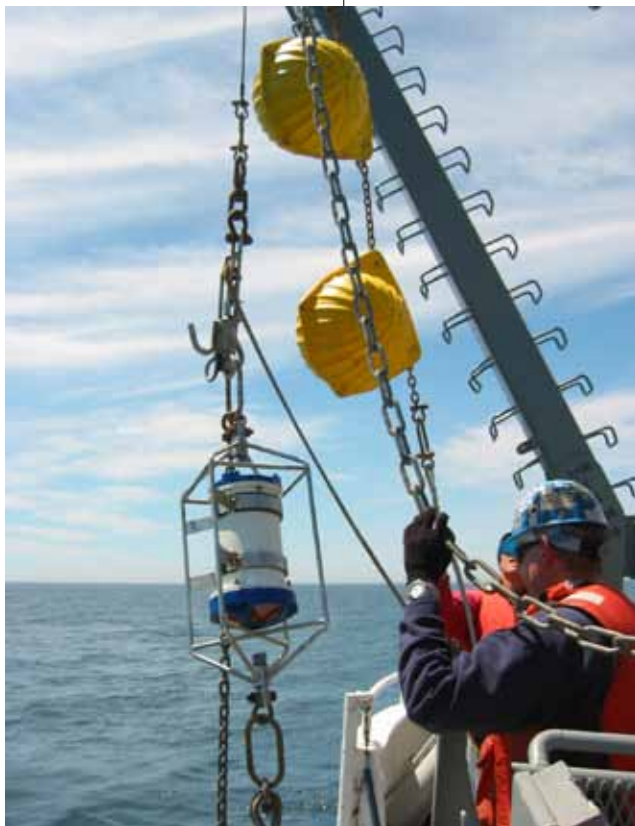
An acoustic Doppler current profiler, for measuring subsurface currents, goes over the stern as part of an oceanographic mooring. Subsurface floatation is provided by the yellow “hard hats” containing glass balls.
